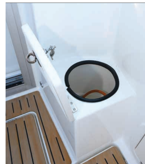
Storage for LPG tank
