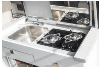
Galley with pressure water, LPG stove, refrigerator and microwave
