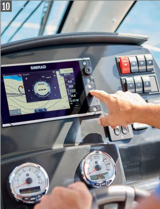
Integrated helm with SmartCraft instrumentation, mounting area for 9" GPS/Chart Plotter
