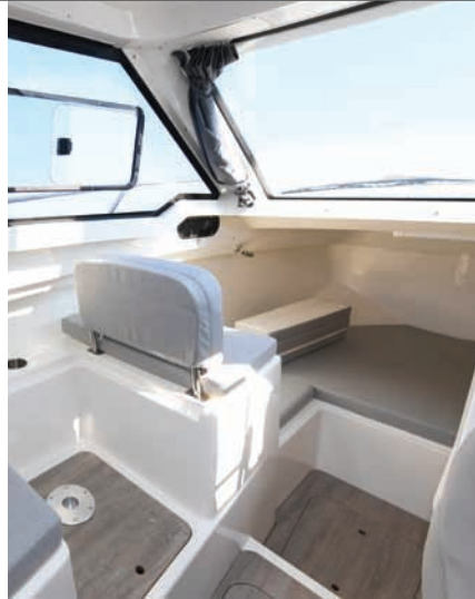
20 Double co-pilot seat with bi-directional seat backrest
