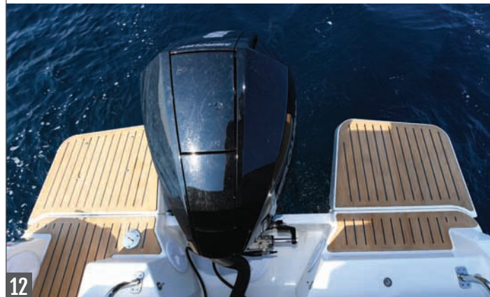
Large swim platforms and motor well step for easy access to both sides of transom
