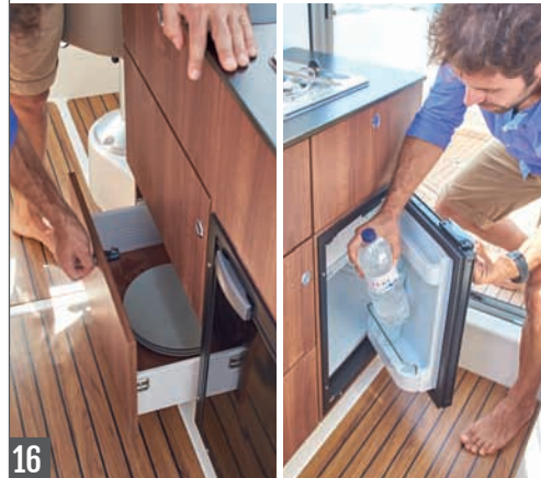
Galley with pressure water with LPG stove and refrigerator*
