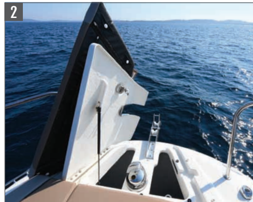
Anchor storage and step-out area via the bow
